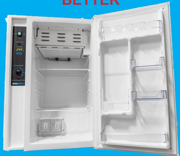
Units are equipped with a hermetically sealed compressor, a circuit breaker to protect from electrical overload, and an easy-to-clean, fully insulated chamber. Gentle, continuous forced-air circulation ensures temperature uniformity and reproducible test conditions. The Refrigerated Incubators also include an independent over-temperature safety controller, 3 adjustable shelf positions, two interior outlets to allow the use of shakers, stirrers, roller bottles, or other apparatus.
