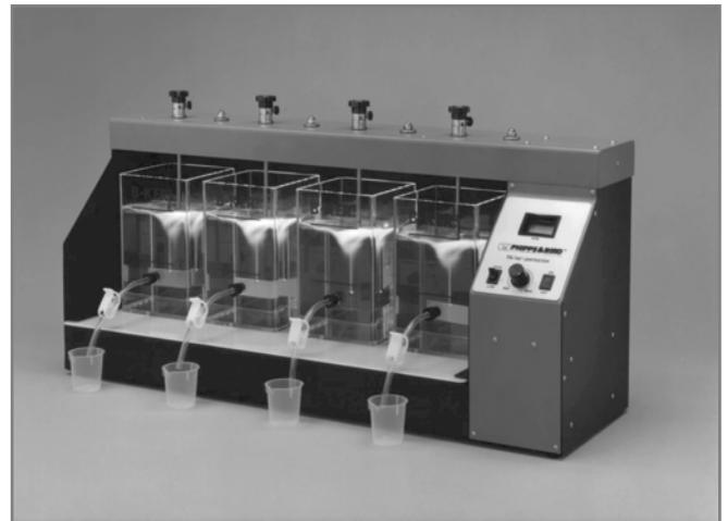
Each JarTester comes complete with your choice of B-KER<sup>2</sup>® square, acrylic, 2-liter testing jars or 1-liter round glass beakers. All Phipps & Bird JarTesters are available in 120V, 60 Hz or 220V, 50/60Hz and are covered by a one-year manufacturer's warranty.
