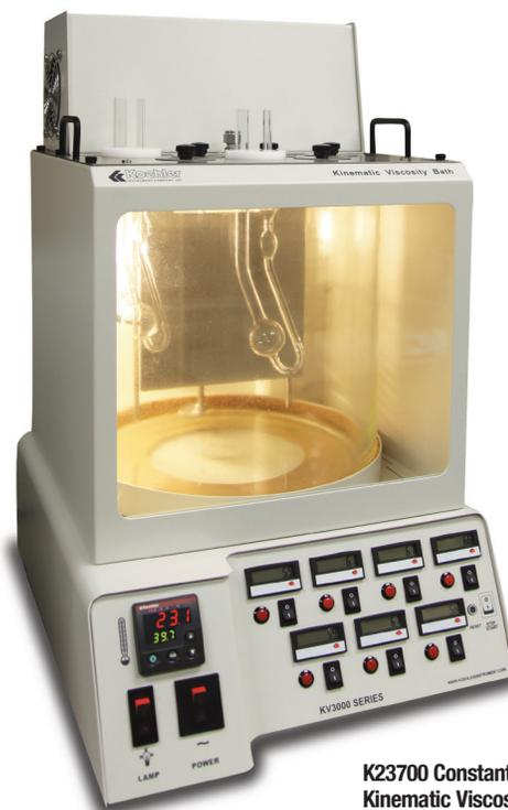
**K23700 Constant Temperature Kinematic Viscosity Bath (KV3000)**
