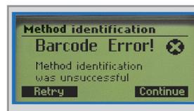
**Barcode Error:** The instrument cannot identify the vial's bar code or the vial has no code.
