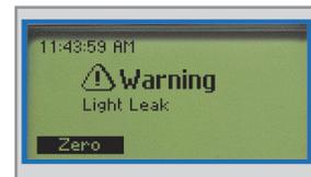
**Light Leak:** There is too much light entering the cell for accurate measurement.
