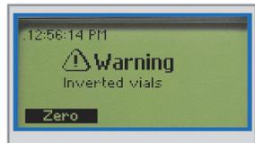
**Inverted vials:** The sample and the zero vials are inverted.
