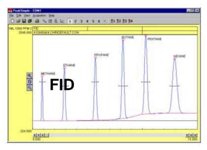
A 1mL sample of 1000ppm C<sub>1</sub>-C<sub>6</sub> hydrocarbons was separated with an Educational FID GC to produce this chromatogram. The FID response is linear and reproducible. Stable from day to day, the FID is not susceptible to contamination from dirty samples or column bleed. The FID is the preferred detector for general hydrocarbon analysis.
