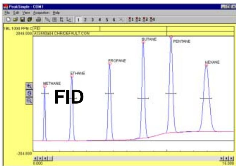
A 1mL sample of 1000ppm C<sub>1</sub>-C<sub>6</sub> hydrocarbons was separated with an Educational FID GC to produce this chromatogram. The FID response is linear and reproducible. Stable from day to day, the FID is not susceptible to contamination from dirty samples or column bleed. The FID is the preferred detector for general hydrocarbon analysis.
