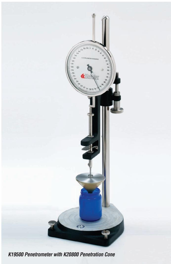
*K19500 Penetrometer with K20800 Penetration Cone*
