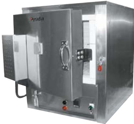
**LONG SERVICE LIFE & EASE OF MAINTENANCE** The specially designed grooved bricks optimize heat transfer and fully support the FeCrAl heating elements for maximum life expectancy. The "open coil heating elements" are easily accessible for maintenance.
