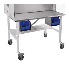
**5328800—Storage Bin Kit.** Organization for syringes, IV bags and other consumables. Mount underneath the work surface of the Nexus. Kit includes one bin and bracket with mounting hardware. Internal bin dimensions: 10" w x 7" d x 6" h (25.4 x 17.8 x 15.2 cm). Compatible with Nexus telescoping and hydraulic base stands. **Installation required**. Shipping weight 7.0 lbs. (3.2 kg)
