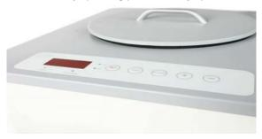
• A large-volume open reservoir allows easy filling and supports cold trap experiments
