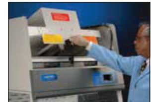
**Convenient, front-accessible filter replacement.** The gas spring-assisted clamping mechanism opens effortlessly and applies uniform pressure across the top surface of the filters for leak-proof, one-step filter replacement.
