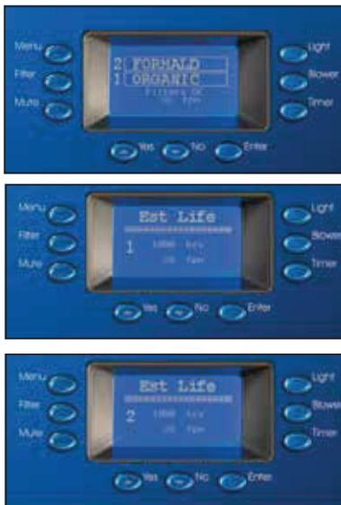
Above: 4' Paramount Ductless Enclosure 6963401 is shown with Work Surface 3909902 and Protector Standard Base Cabinet 9900000. Work Surface, Base Cabinet and filters are sold separately. At left: Three screens alternate on the LCD display: filter types and status, estimated filter life for the bottom filter(s), and estimated filter life for the top filter(s). All three screens display face velocity.
