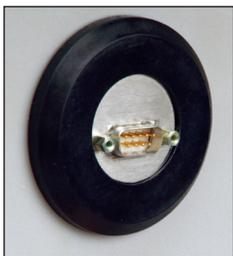
Provides a leak-tight connection for data transfer to a customer-supplied printer or computer located outside the glove box. Includes sealed 9 pin connector (D-subminiature with male pins on one side and female pins on the other) and 10' cord. **Requires installation and drill hole.** Installation Kit 5241100 is recommended. Shipping weight 1 lb. (0.5 kg)
