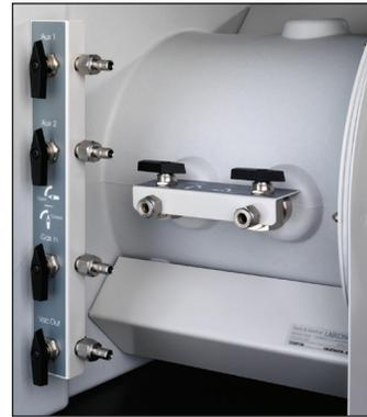
Includes six each manual ball valves, pressure relief valve, compression fittings, hose connector fittings, holesaws, O-rings and nuts to add four service valves to the main chamber and two service valves to the transfer chamber. Two of the valves on the main chamber and two on the transfer chamber may be used for evacuating and filling. The remaining two on the main chamber are for drying train connections. **Requires installation.** Precise Controlled Atmosphere Glove Boxes include six manual
