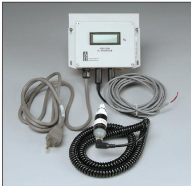
Oxygen Monitor measures percent of oxygen inside the glove box using a chemically resistant electrochemical sensor. Front LCD panel displays percentage from 0.1 to 100%. Includes interconnecting sensor cable and power cord for connection to the glove box's interior electrical receptacle. An "O" ring is
