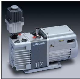
For evacuating the main chamber and/or transfer chamber. Ultimate vacuum (total pressure) is  $2 \times 10^{-3}$  mBar (1.5 micron). Consist of on/off switch; two inlet adapters (1/2" and 3/4" OD); mode selector with High Vacuum and High Throughput positions; and gas ballast with closed, low flow and high flow positions. Single phase, direct drive motor, totally enclosed and fan cooled.
