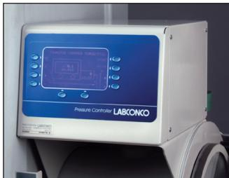
For use with Protector Controlled Atmosphere Glove Boxes without Automatic Pressure Controller. Easily reduce glove box oxygen and moisture levels by automating the evacuation/purge process via LCD display. Automatically regulate pressure and vacuum within the main chamber and transfer chamber by automating evacuation/fill cycles.
