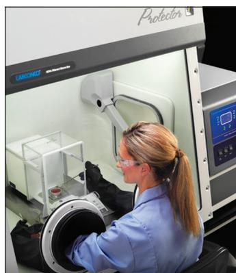
The glove box was tested at various blower speeds and under typical laboratory conditions. No efforts were made to isolate the glove box from foot traffic and laboratory equipment operating in the area. Results were excellent. The analytical balance readings remained stable to five decimal places.
