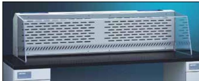
Fume Adsorbers are designed for light duty applications involving organic solvents, formaldehyde, ammonia or low molecular weight amines. Fume Adsorbers use carbon filtration to trap vapors so that safe, filtered air is returned to the laboratory. No outside ducting is required. These portable, low profile enclosures fit easily on counter-tops with overhanging cabinets and are available in two widths.
