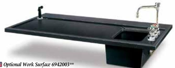
**Optional Work Surface 6942003\*\*** of solid black epoxy is corrosion and stain resistant and dished to contain spills. Includes a 10" x 14" x 6" deep molded epoxy sink; corrosion-resistant, chrome-plated gooseneck fixture with vacuum breaker and two faucet controls. A retractable hose with spray nozzle speeds clean up. A Solid Epoxy Work Surface without sink is also available. Contact Labconco for ordering information.
