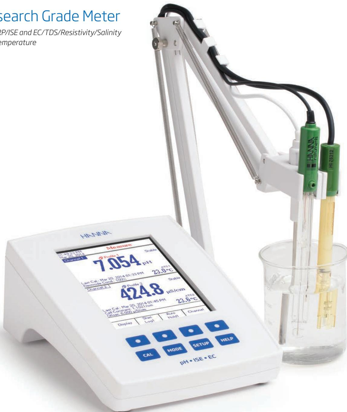
The HI5522 is an advanced research grade benchtop pH/ORP/ISE and EC/TDS/Salinity/Resistivity meter that is completely customizable with a large color LCD, capacitive touch keys, and USB port for computer connectivity.
