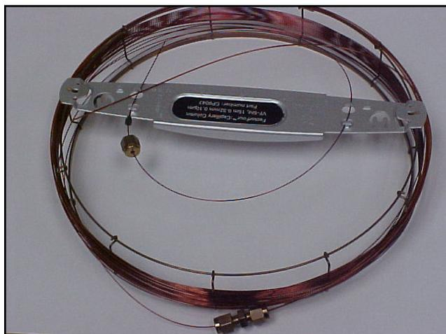
SRI currently (September 2008) uses the Restek MXT-BiodieselTG column. Restek part# 562551-2731
