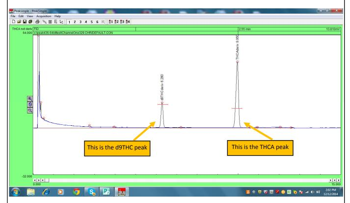
can the proper decarboxylation of the ingredients be confirmed prior to mixing it in to the final product, but the final product's THC content can be determined before sale or distribution. Even if a "certified" lab must be used by state law to measure the THC levels, it is helpful to be able to make quick in-house tests during the production process.
