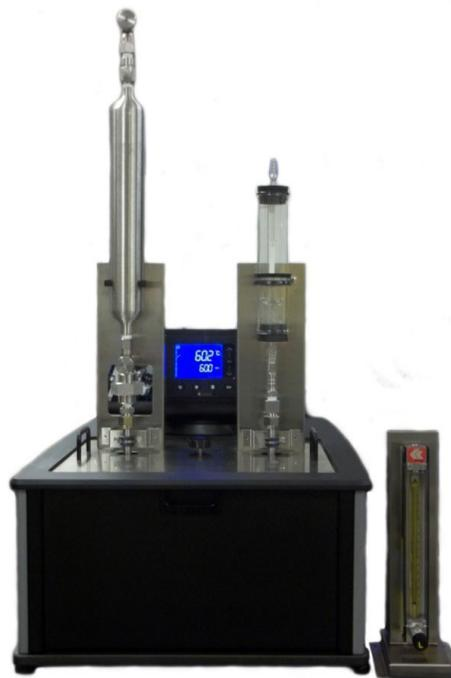
K48200 Hydrogen Sulfide Apparatus
