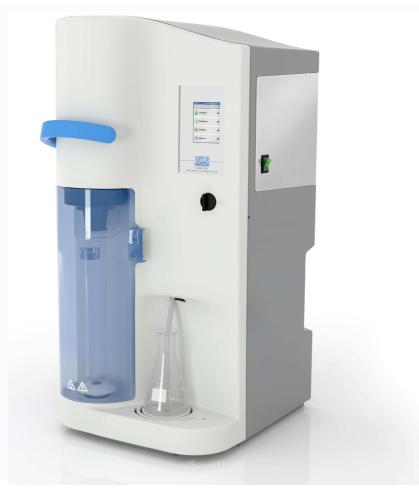
The UDK 139 Semi-Automatic Distillation Unit is designed to perform nitrogen and protein content analysis according to the Kjeldahl Method (TKN) in the Food & Feed industries and several other applications in environmental control (phenols, nitrogen in water, sludge, soil and lubricant) and also in the chemical and pharmaceutical industries after having digested the sample accurately.
