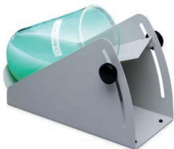
**7369700—Slant Freeze Flask Holder.** Slant freezing increases the surface area to volume ratio, maximizing freeze drying rate. Angle is manually adjustable from 5° to 35°. Powder-coated steel. 10.4" w x 4.5" d x 6.7" h. Shipping weight 3.5 lbs. (1.6 kg)
