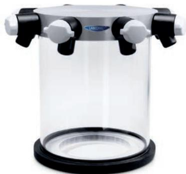
**Clear Chambers with Valves.** For interior view of product shelves and glassware connection. Includes acrylic base, anodized aluminum lid, and eight neoprene valves with molded plastic knobs. For 1/2" and 3/4" flask adapters. 8" dia. opening and cap for 3" dia. attachment port.
