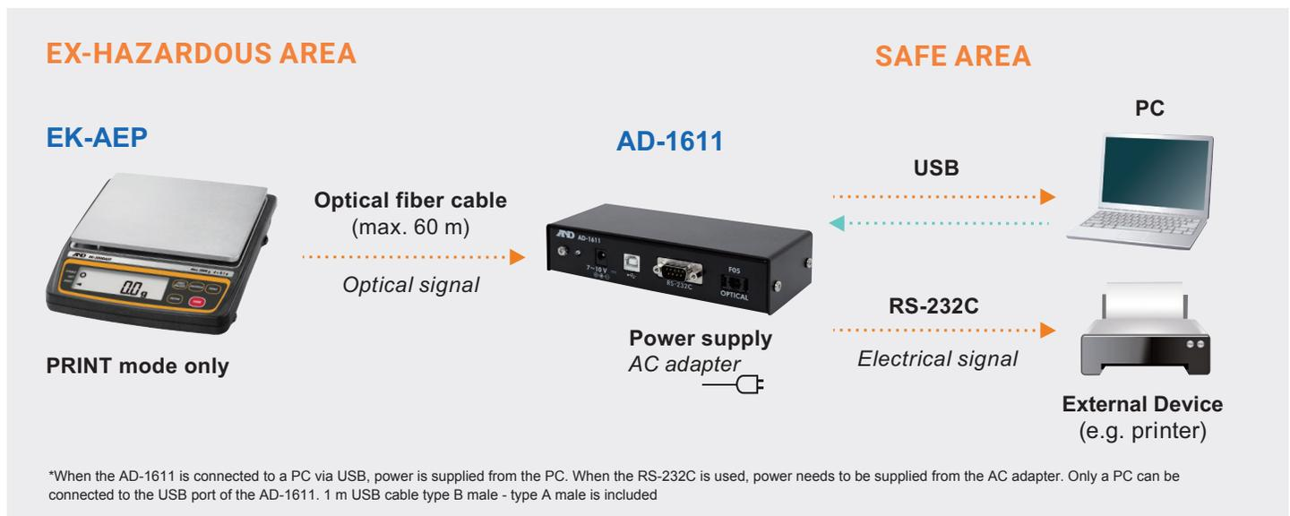
\*When the AD-1611 is connected to a PC via USB, power is supplied from the PC. When the RS-232C is used, power needs to be supplied from the AC adapter. Only a PC can be connected to the USB port of the AD-1611. 1 m USB cable type B male - type A male is included
