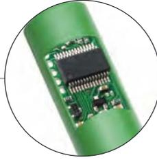
Stored pH calibration information includes: calibrated buffers, date, time, offset and slope characteristics of the electrode. Conductivity calibration information includes: calibrated conductivity standards, date, time, and cell constant of the sensor. Dissolved oxygen calibration information includes: standards used for calibration, date, time, altitude and salinity correction.
