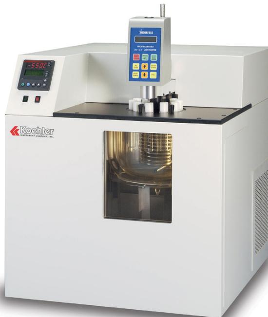
K34715 Programmable Brookfield Viscosity Liquid Bath System (BVS5000)
