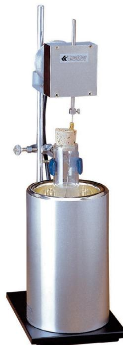
K29750 Freezing Point Apparatus
