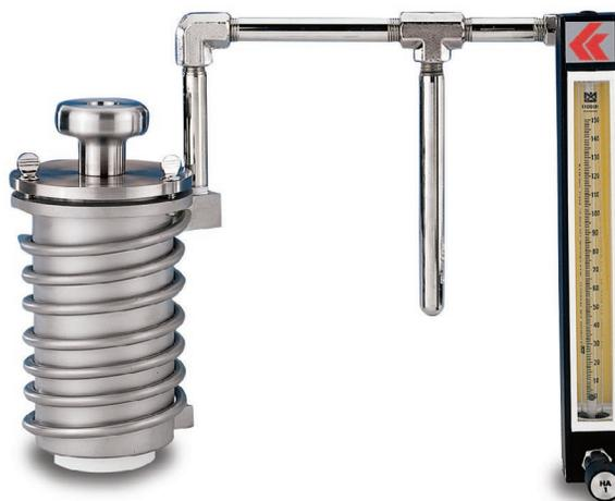
K29500 Evaporation Test Cell
