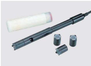
Palarographic DO Probe with automatic compensation for temperature and salinity
