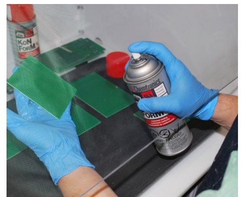
Close-up of operator spraying conformal coating under the 30" DSH.
