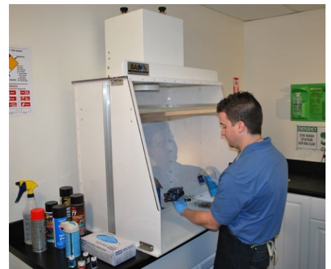
30" DSH provides fume control for a variety of aerosol spray applications.
