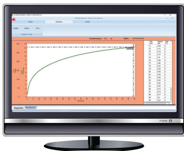
Oxidata® software automatically tracks measured data in real-time and calculates the endpoint of RPVOT (RBOT)/TFOUT test methods
