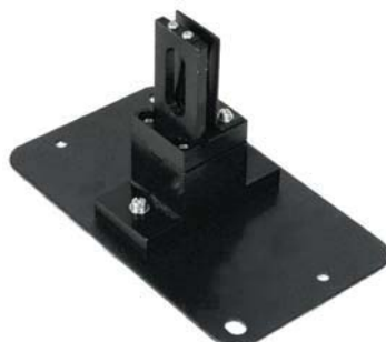
Cat. No. 18900339 solid sample holder (ø1.5-3mmø1 position)
