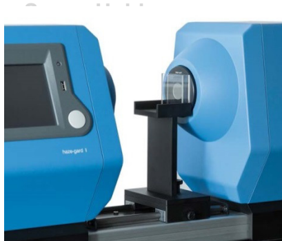
Liquids are best measured using cuvettes and the cuvette table.
