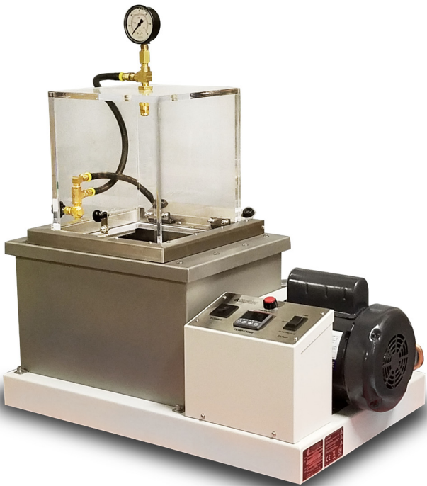
K18201 Digital Water Spray Off Tester
