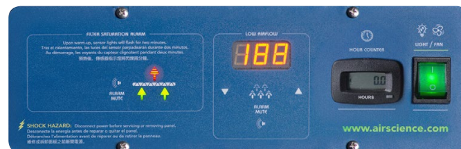
FSA/Autocal Control Panel
