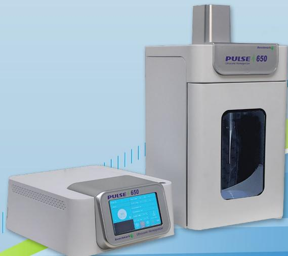
Like the smaller Pulse 150™, the Pulse 650™ utilizes ultrasonic waves and cavitation to disrupt cells, shear DNA and create emulsions. With up to 650 watts of power, samples from 0.1ml to 500ml can be processed. Pulsed operation, power ratios and other operating parameters are easily set using the large touch screen. Alarms alert the user to over temperature, over/no load and expiration of time.
