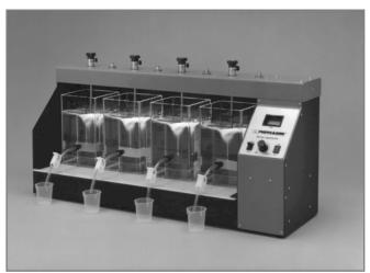
stirrer does not erase the programmed information. The stirrer may be run independently in any one of the memories, continuously at a selected speed or sequentially through the memory banks. Running it in 'sequential mode' permits automatic transitioning from a fast mix/short run to a slow mix/long run, or any combination or speeds and times desired to replicate actual plant conditions and operation.
