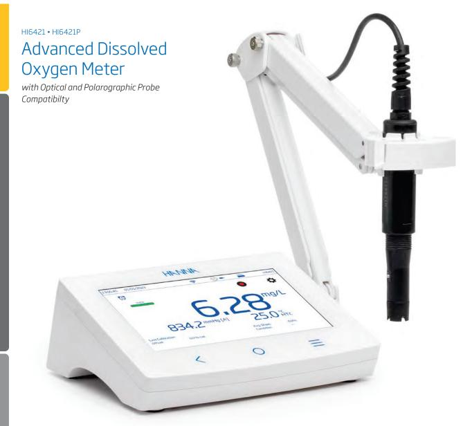
HI6421 and HI6421P are streamlined benchtop meters with a large touch screen display, comprised of a housing and an integrated module designed for fresh and saltwater measurements of dissolved oxygen.
