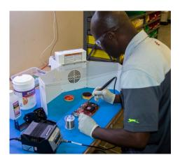
The Winged Sentry with lid helps protects the operator from harmful soldering fumes.
