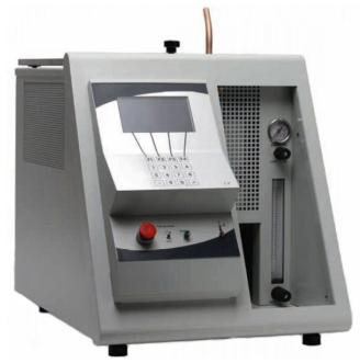
K41091 Micro Carbon Residue and Ash Tester
