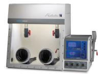
The **Protector Combination Glove Box** functions as a filtered glove box with the added ability to be switched to a controlled atmosphere box as needed. See pages 13-14 for more information.
