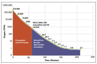
In this test, the AtmosPure Re-Gen Gas Purifier reduced the oxygen level inside the Protector Stainless Steel Controlled Atmosphere Glove Box to 0.7 ppm (0.00007%)
