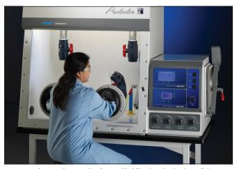
Protector Combination Glove Boxes have features of both filtered ventilated and controlled atmosphere glove boxes. Two internal valves allow the box to be converted from filtered mode to controlled atmosphere.
