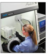
tested at various blower speeds and under typical laboratory conditions. No efforts were made to isolate the glove box from foot traffic and laboratory equipment operating in the area. Results were excellent. The analytical balance readings remained stable to five decimal places.
