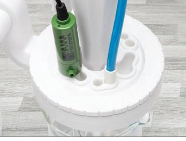
The electrode holder is easy to flip to gain added height.
