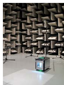
ISO 3744 anechoic test
