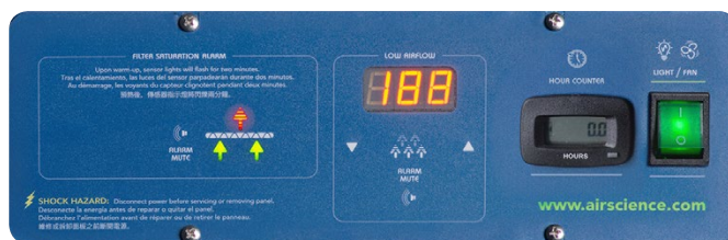
FSA/Autocal Control Panel
