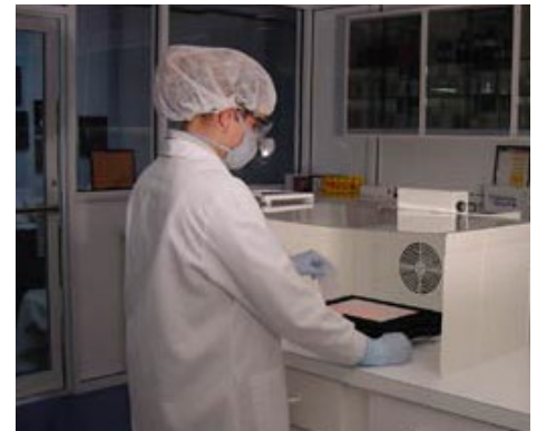
The Model 300 Winged Sentry with lid extracts most of the fumes and particulate for a variety of laboratory and medical applications.
