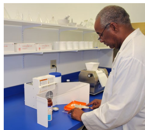
The Model 200/225 Winged Sentry with lid extracts most of the airborne particulate for pharmaceutical applications.
