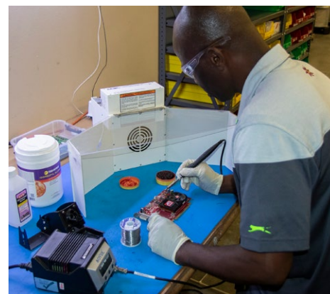
The Winged Sentry with lid helps protect the operator from harmful soldering fumes.
