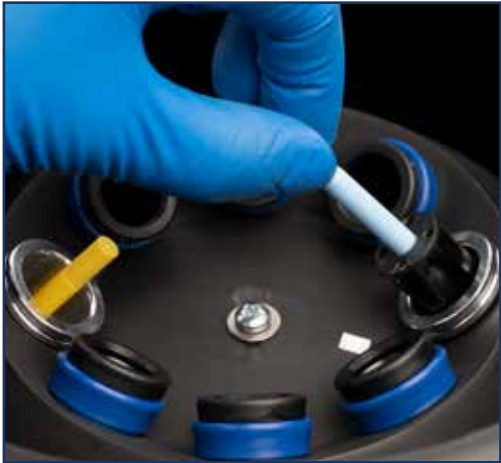
Insert the carrier in the metal tube sleeves.
