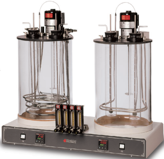
K43092 Dual-Twin Foaming Characteristics Apparatus
