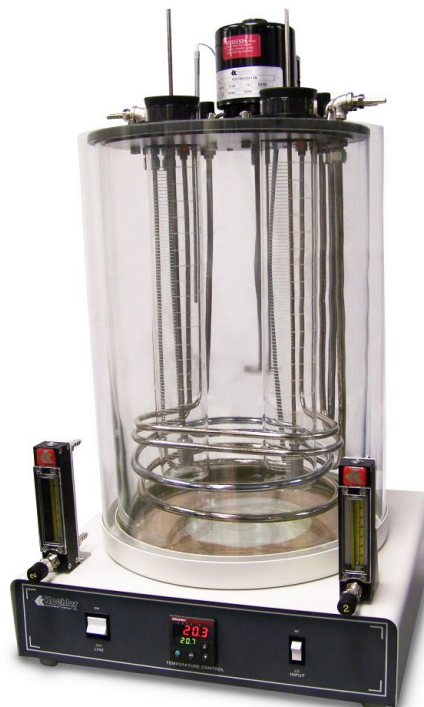
K43041 Sequence IV Liquid Foaming Characteristics Apparatus
