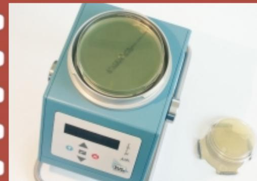
Set the Total Volume of air to be processed, the Delay to start and the Rotation speed for the Petri dish.
