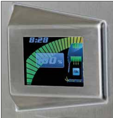
Bar graph displays percent of HEPA filter life remaining
