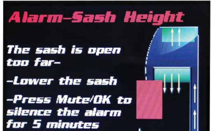
Various alert and alarm messages may be displayed and provide clear feedback and instruction.
